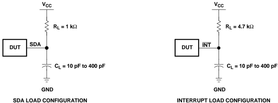
Figure 4. Load Circuits
