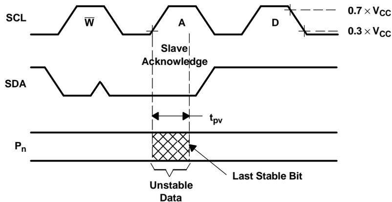
Figure 3. I<sup>2</sup>C Write Voltage Waveforms
